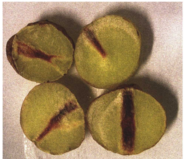
Figure 2.33. A selection of four raw potato chips with diameter about 30 mm and thickness 4 mm, after partial drying in a microwave system providing dominant TM-polarised modes with no load movement. Note that the orientations are changed in the photo. – Courtesy of SIK, Sweden.
