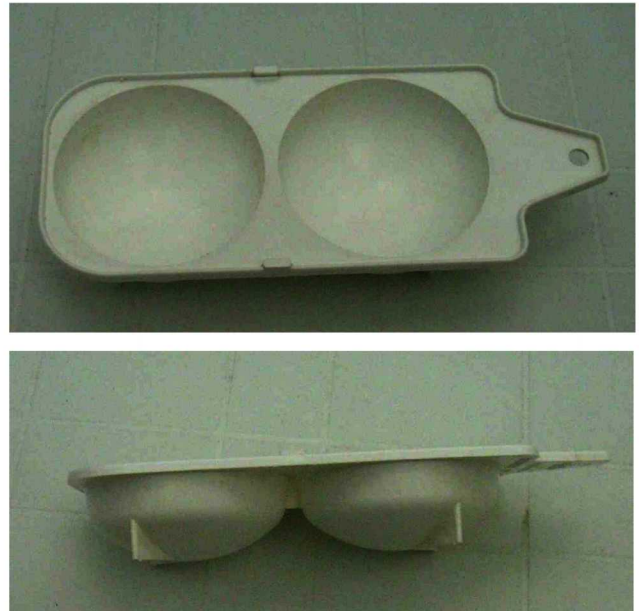
Figure 2.29. A commercially available microwave oven egg cooker. The spherical segment-shaped “holes” are 78 mm in diameter and 30 mm high; a normal chicken egg fills up to about 23 mm.
