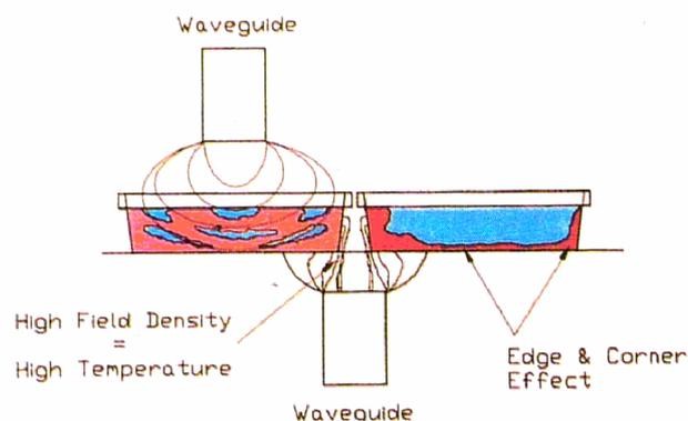
**Fig.3** Illustration of simple waveguide applicators for food pack pasteurisation (from Berstorff, 1992). In order to overcome the problems with edge overheating (and also surface waves, as seen in the illustration), applicators were energised only for short intervals when at pack centres.
