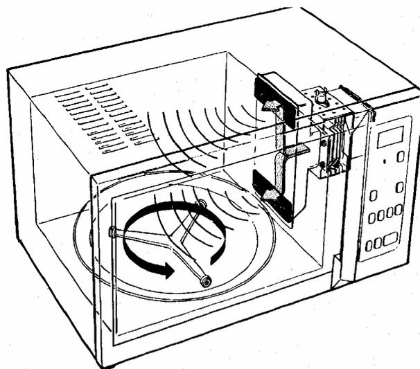
**Fig.2** Illustration of the Whirlpool *DES* system.
