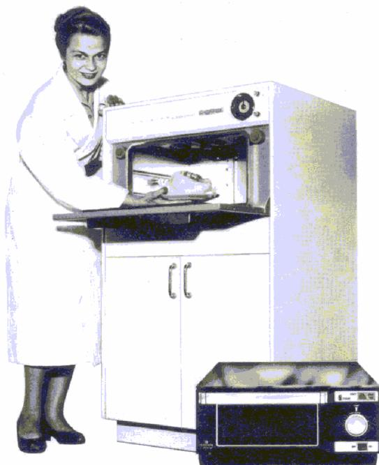
**Fig.1.** Two Husqvarna ovens: a 1957 floor-standing unit, and a 1972 commercial 1200 W oven with near-field cavity and the world's first automatic humidity sensing control. Note the choke seal in the old oven (the Schmidt patent).
